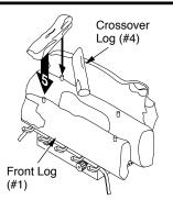
Figure 29 - Installing Crossover Log (#5) (CCL3018PR/PRA and CCL3018NR/NRA Only)
